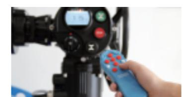
Integration and Intelligent type come with infrared remote control for easy menu access.
